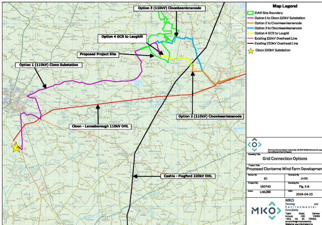
Figure 3-8 Grid Connection Options – Iteration 1
